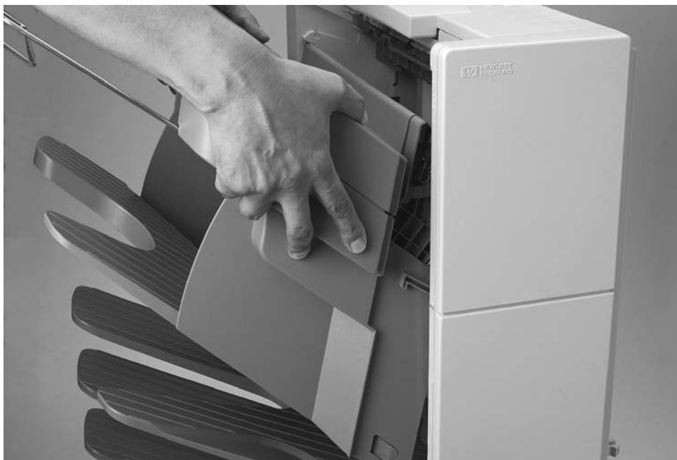
Figure 6-178 Mailbox with Stapler, Stapler Removal or Installation
