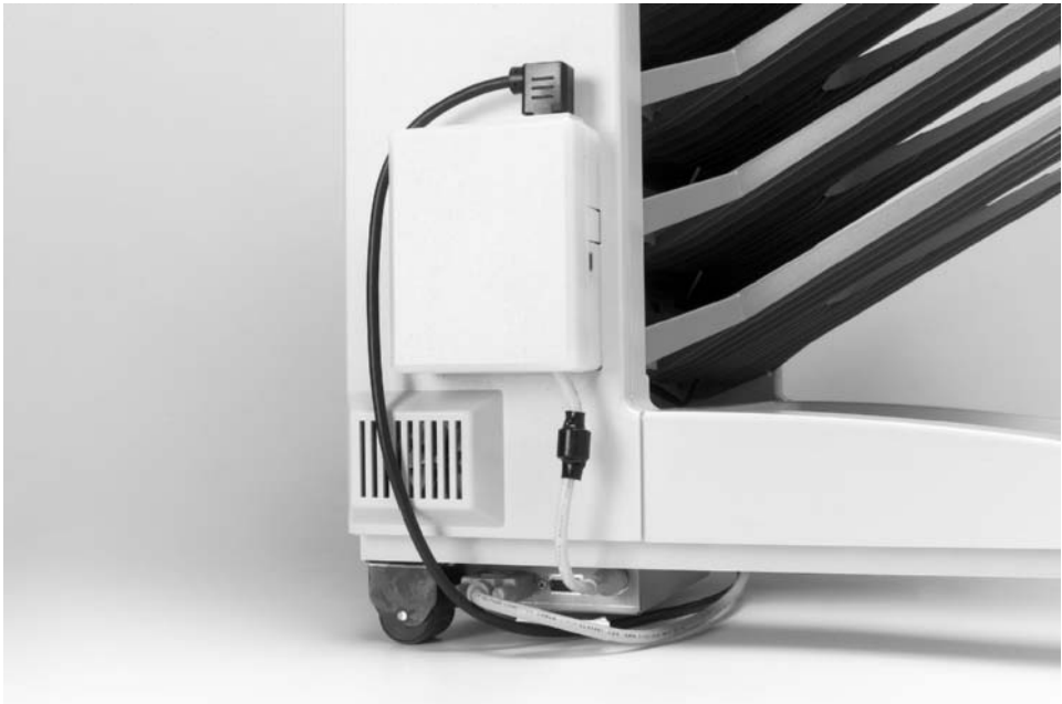
Figure 7-10 8-bin Mailbox Power Supply Test Mode Switch
