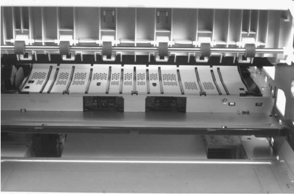
Figure 6-32 Feeder Assembly (2 of 2)
