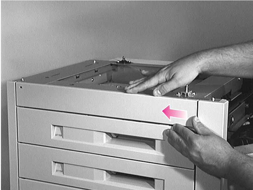
Figure 6-92 Front Top Cover (3 of 3)
